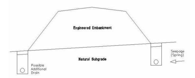
1. The minimum desirable design grade is 1%. For non-corrugated pipes an absolute minimum grade of 0.5% is acceptable.
